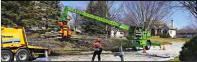
*A specialized telehandler being used to quickly move material into a large chipper.*
